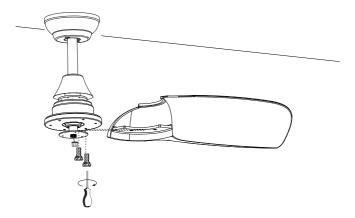
(2) Remove the pre-installed screws. Connect the light kit cable, and then lock the light kit.
