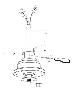
(3) Install in order the yoke cover, Canopy, Hanging Ball on the installed Down rod. slide Hanging Ball down to expose the hole, put the fixing pin into the hole, slide the Hanging Ball up and turn it left and right, let the fixing pin enter the Hanging Ball card slot.
