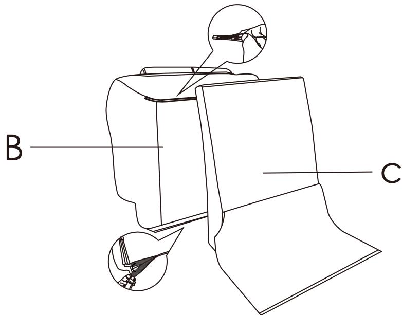
STEP10:Plug the back pad into the seat frame, and then connect the massager line white and white, red and red, black and power lines, and the massage line with the hand controller.
