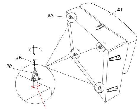
Make sure the wheel is installed in the marked position. Note: the marked position has not yet drilled the screw hole.
