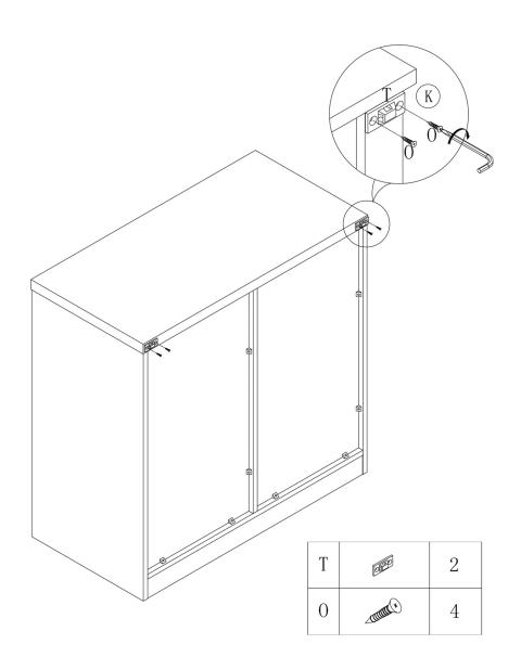
Step 12. Fix metal part T on cabinet back with Screw O.
