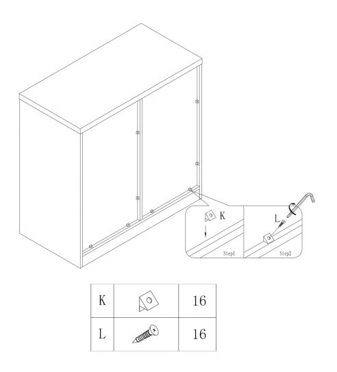
$\label{eq:Step 11.} Step \ 11.$  Fix component K on the cabinet back with Screw L.
