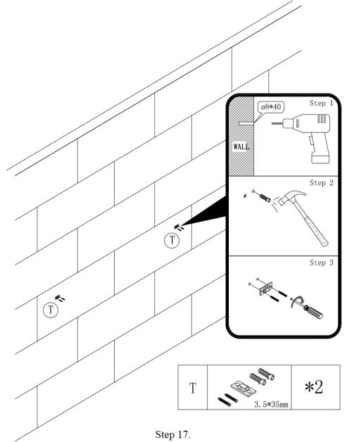
Drill holes( $\phi 8*40$ ) on the wall at proper position with electric drill, Fix T on the wall with hammer and screwdriver.
